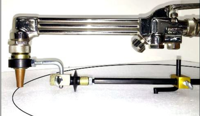
Fig. C Both wheels on one side for trimming or beveling the edges of plate.
